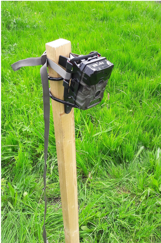
Fig. 2 Modified trail camera for nest monitoring purposes. The upper LED panel was covered by a lightproof film to reduce the flashlight intensity. Two holes (4 mm diameter) are left out: one for a single LED and one for the light sensor. The lower LED panel was turned off
